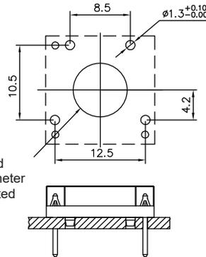
Recommended PCB hole diameter when using listed Piher shafts
