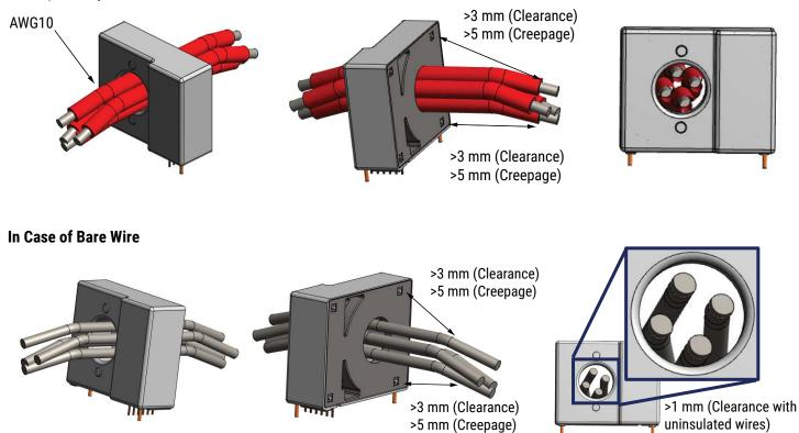
Reinforced insulation, insulation material group III, pollution degree 2, altitude < 5,000 m and overvoltage category II. Please take enough creepage distance between each pin.
