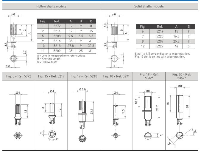
15-mm carbon endless rotation SMD potentiometer
